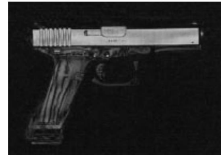
Fig. 6. 350-GHz reconstructed image of a Glock-17 9-mm handgun.
